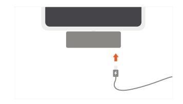
**4** Use the USB 3.0 port to connect external keyboards or thumb drives for photographic media transfer (via DCIM folder).
