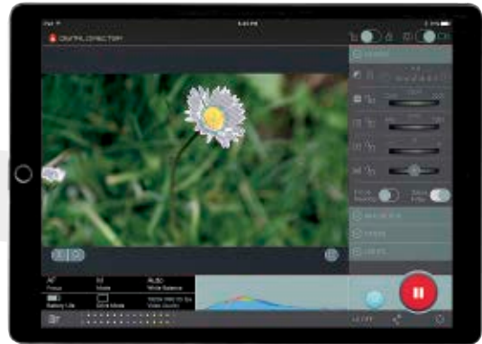
ZEBRA The Zebra filter uses striped patterns to show the over- and/or underexposed areas of the image.
