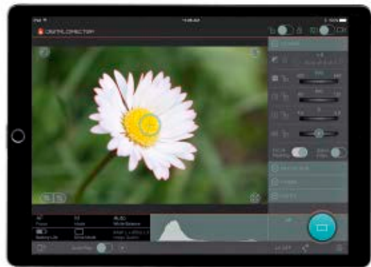
FOCUS PEAKING The Focus Peaking Filter highlights focused profiles on the image (intensity and color profile can be adjusted).
